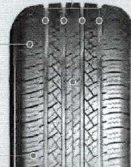
4 circumferential grooves for excellent water evacuation for good wet traction.
